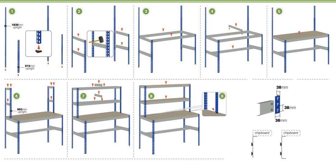
**1.** Attach plastic feet to all 6 uprights, the narrow part of each slot pointing downwards.
