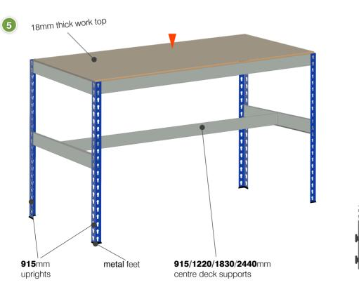
1. Attach plastic feet to all 4 uprights, the narrow part of each slot pointing downwards.
