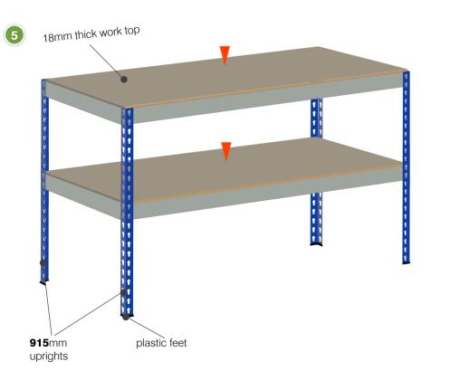
**1.** Attach plastic feet to all 4 uprights, the narrow part of each slot pointing downwards.
