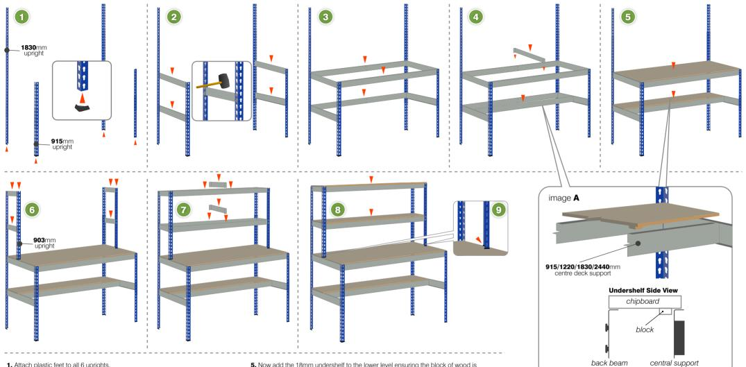
**1.** Attach plastic feet to all 6 uprights, the narrow part of each slot pointing downwards.
